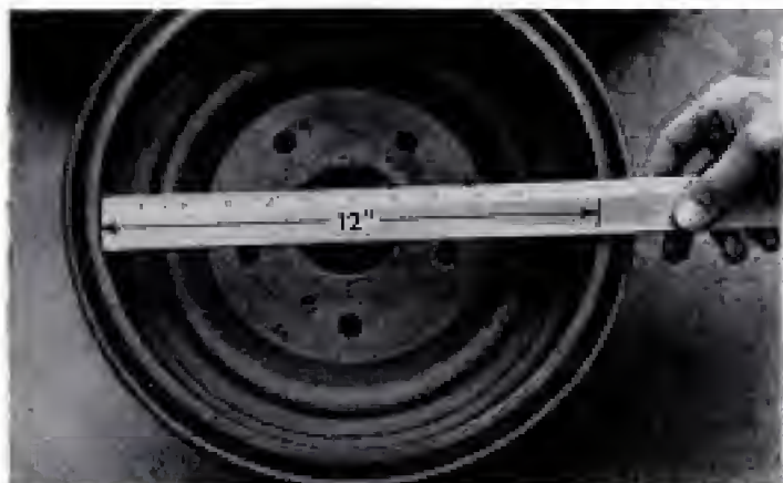
LINCOLN increased brake-drum diameter to 12 inches (1953's was 11), reducing braking effort 25 percent
